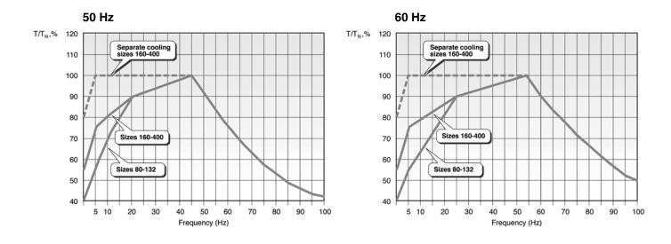
Figure 6. Non-sparking motors Ex nA, cast iron (type M3GP) and aluminium dust ignition proof motors (DIP/Ex tD T125°C), nominal frequency of the motor 50/60 Hz
