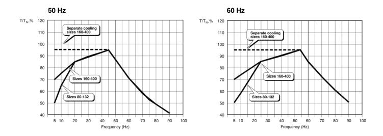
Figure 8. Non-sparking motors Ex nA, cast iron dust ignition proof motors (DIP/Ex tD); nominal frequency of the motor 50/60 Hz
