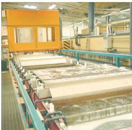
Automatic hot-dip galvanizing plant.
