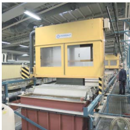
Automatic pre-treatment of enclosures before powder coating.
