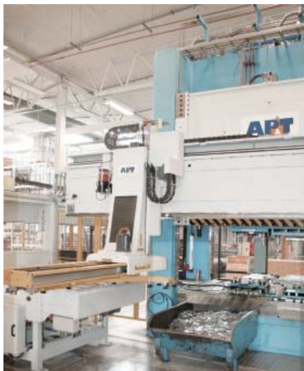
Fully-automatic plant for pressing, punching and bending of metal plates.
