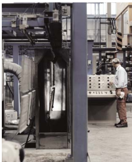
Powder coating of foundation parts.
