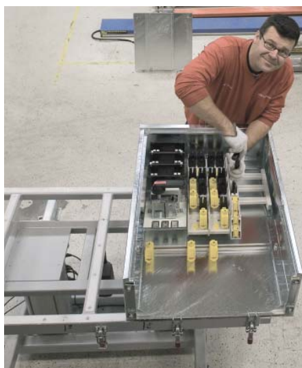
Assembly of distribution boards.
