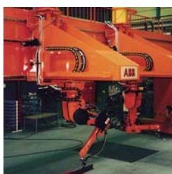
Welding robot equipped with nylon chains.
