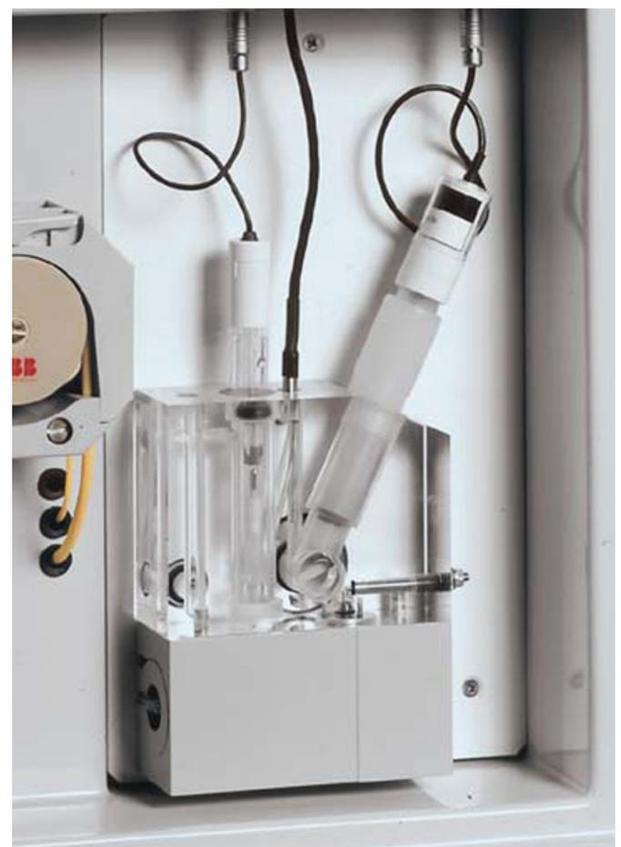
Multi-channel Peristaltic Pump and Sensor Flow Cell
