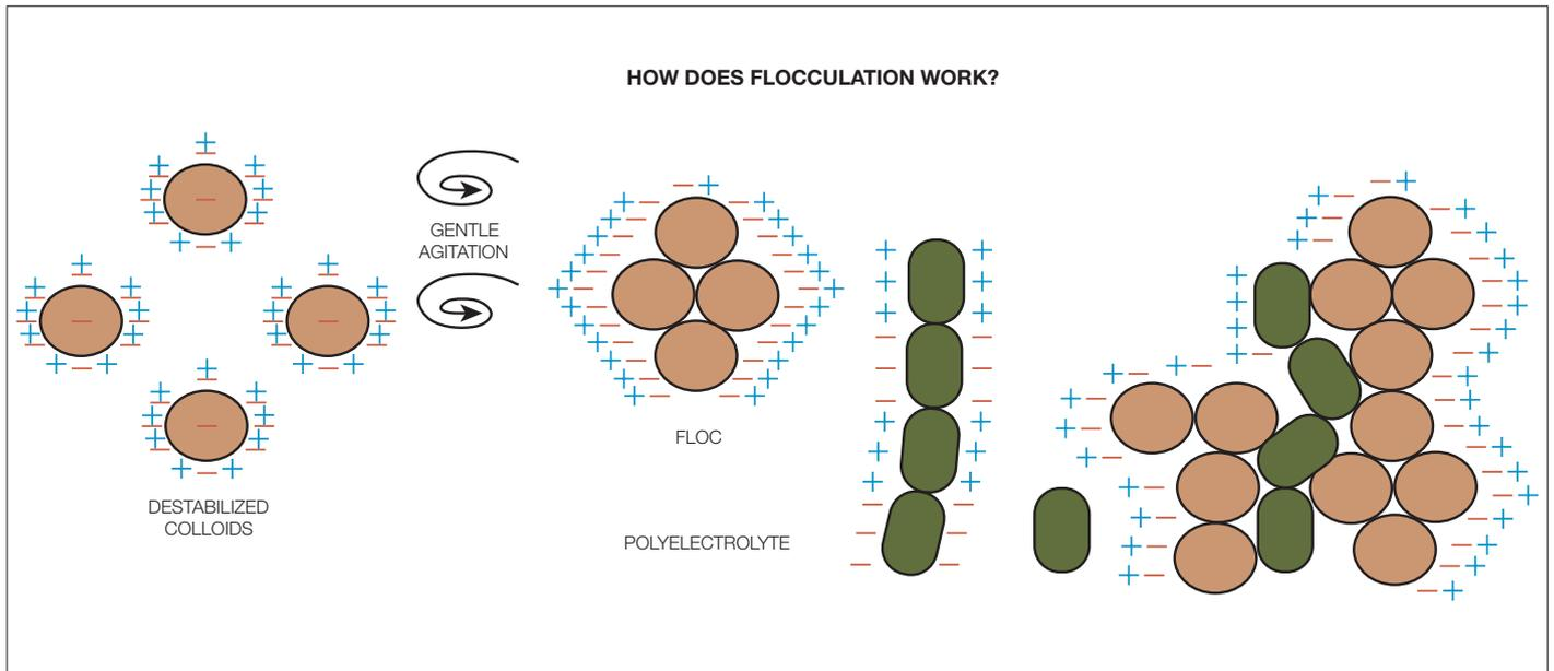
Fig. 4 – diagram showing the flocculation process
