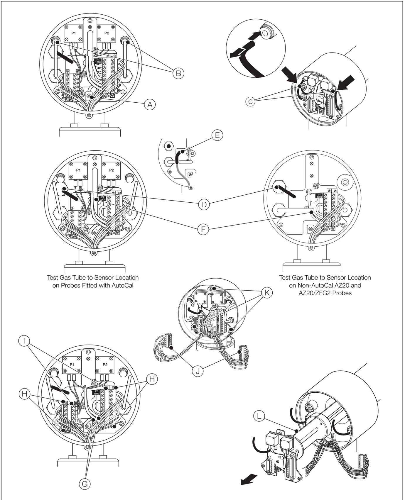
Fig. 5.10 Removing the Heater Assembly
