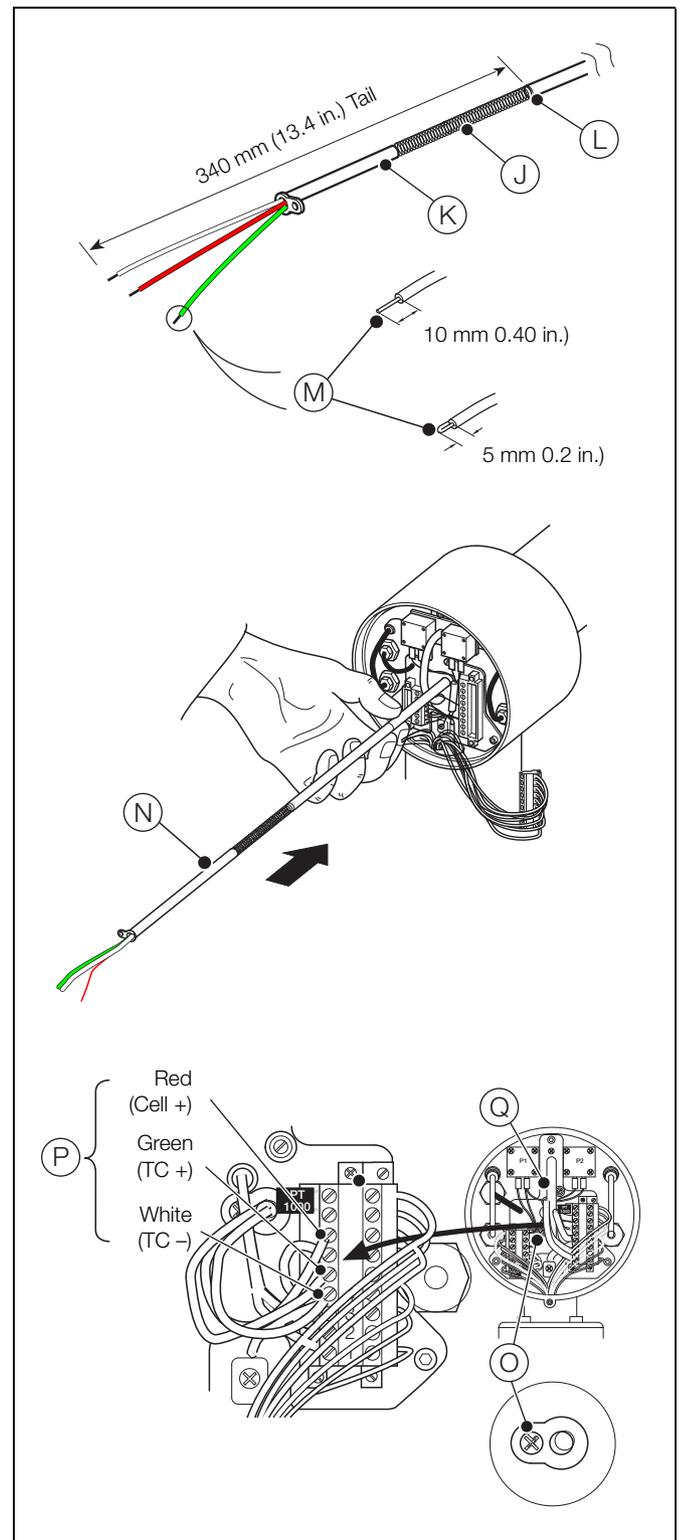
Fig. 5.9 Fitting a New Thermocouple / Electrode Assembly
