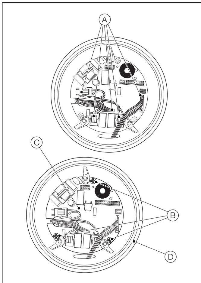
Fig. 6.3 Removing the Backplane from an Integral Transmitter
