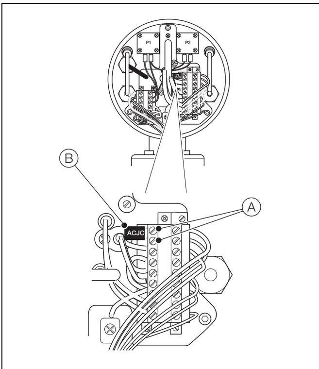
Fig. 5.20 Removing / Replacing the PT1000 Sensor
