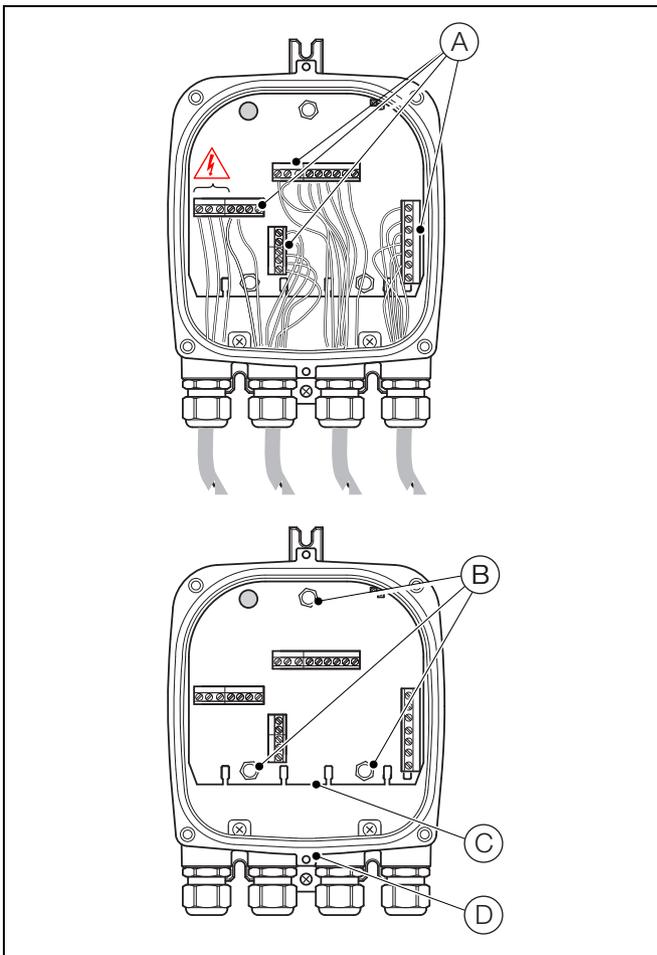
Fig. 6.5 Removing the Backplane from a Remote Transmitter
