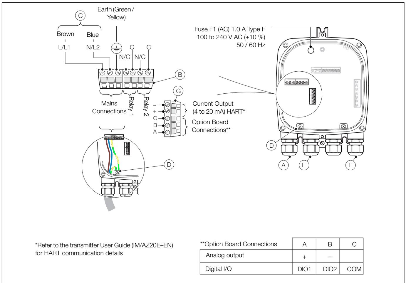
Fig. 6.8 Remote Transmitter – Power Supply and Output Connections
