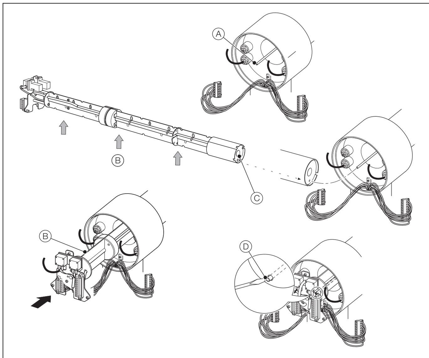
Fig. 5.13 Fitting the Inner Assembly into the Probe Body
