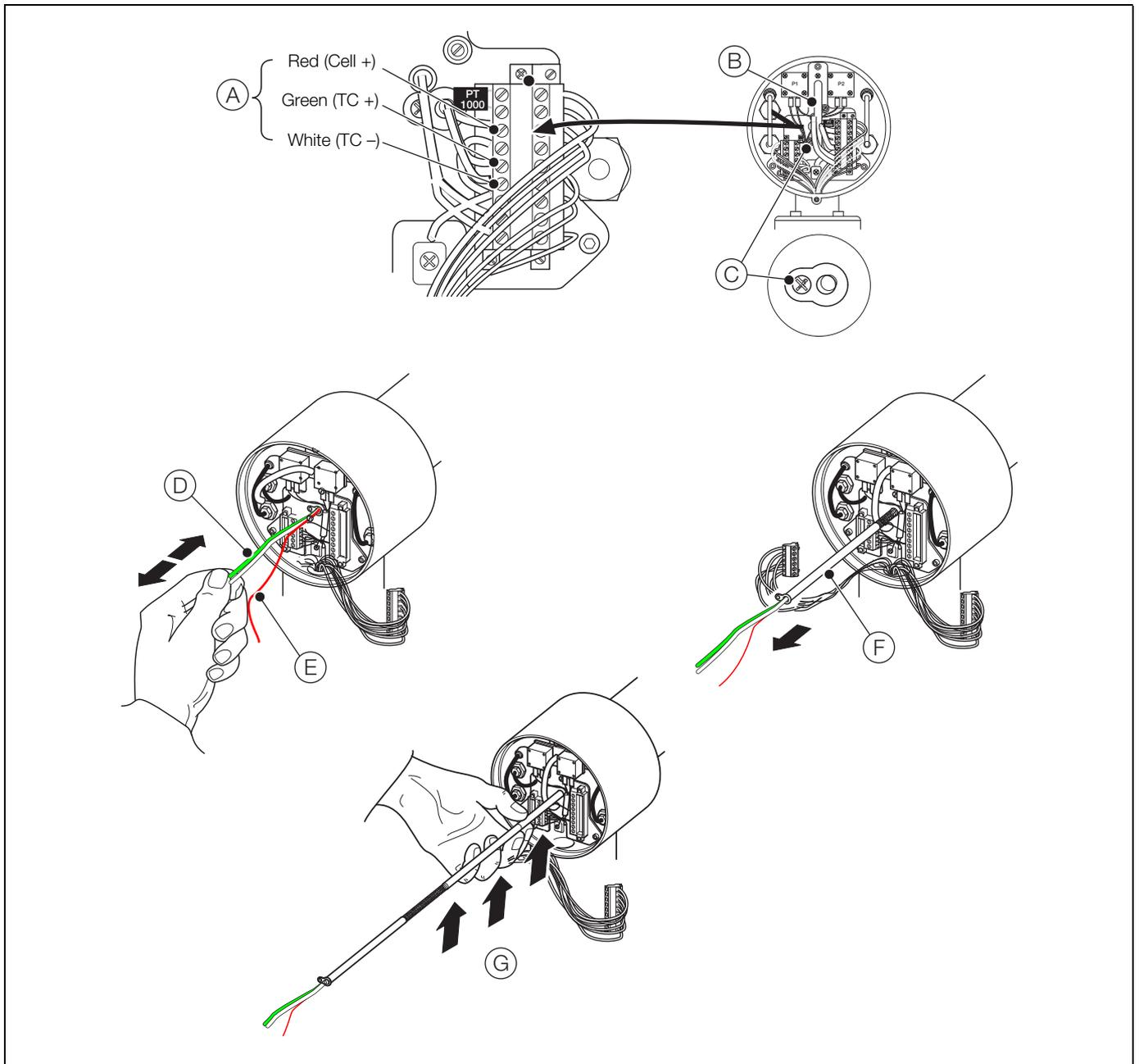
Fig. 5.7 Removing the Thermocouple / Electrode Assembly
