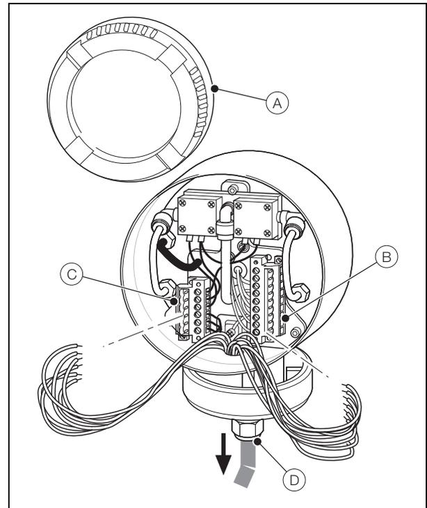
Fig. 5.2 Disconnecting a Remote Probe
