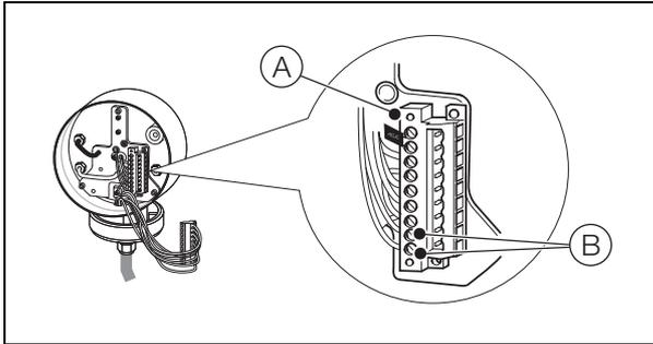
Fig. 3.3 Heater Connections
