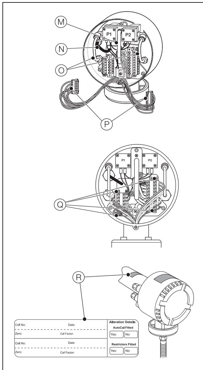
Fig. 5.18 Connecting the Gas / Air Tubes and Recording Commissioning Details
