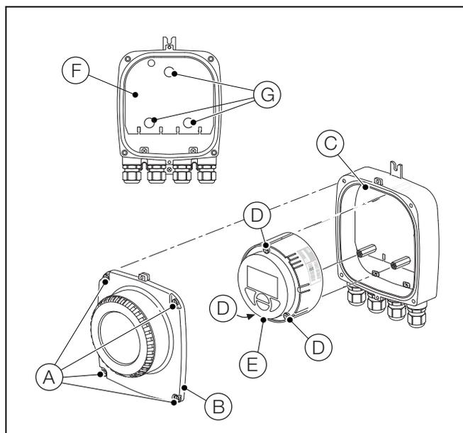
Fig. 6.1 Replacing the Cartridge on a Remote Transmitter
