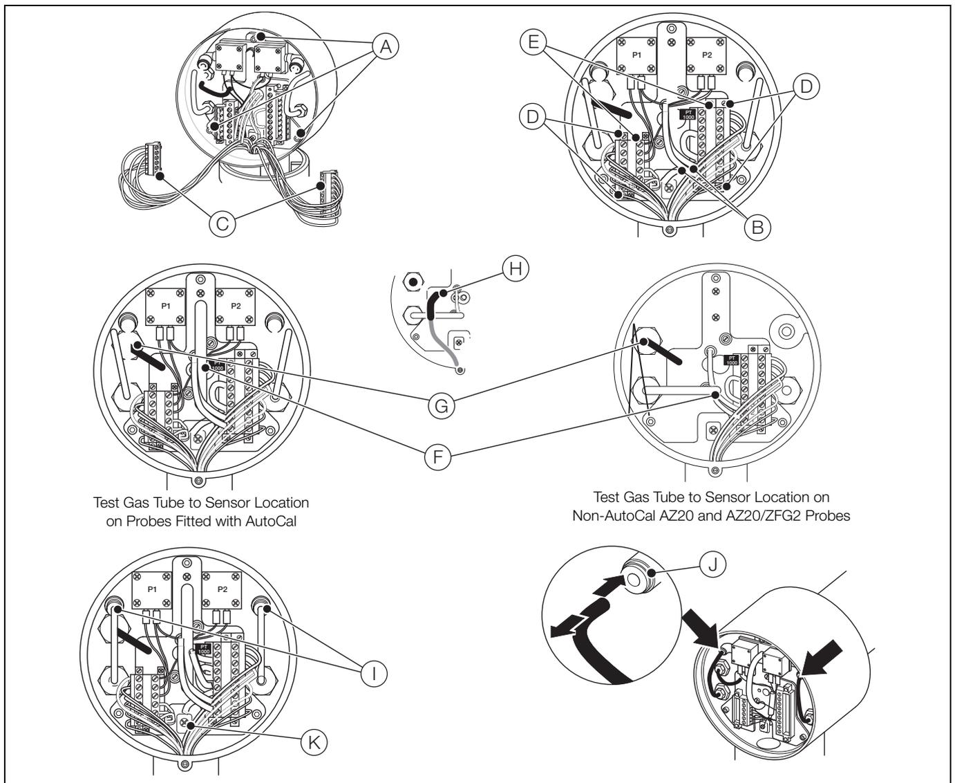
Fig. 5.14 Securing the Heater Assembly and Making Connections
