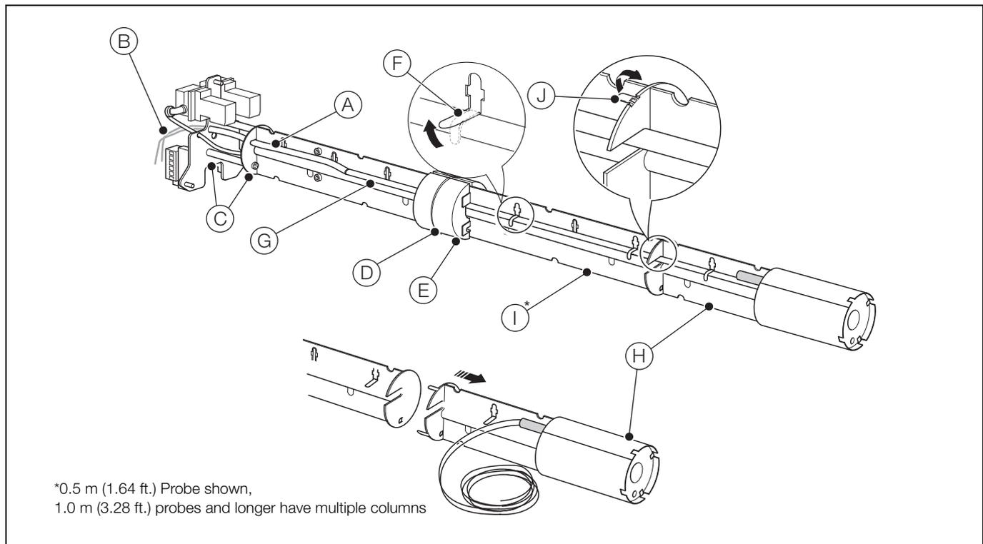
Fig. 5.11 Dismantling the Existing Heater Assembly
