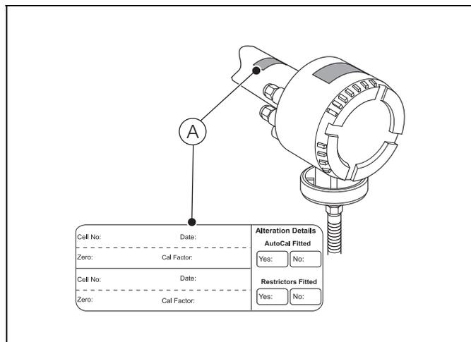
Fig. 5.5 Commissioning Label Details and Location on Probe
