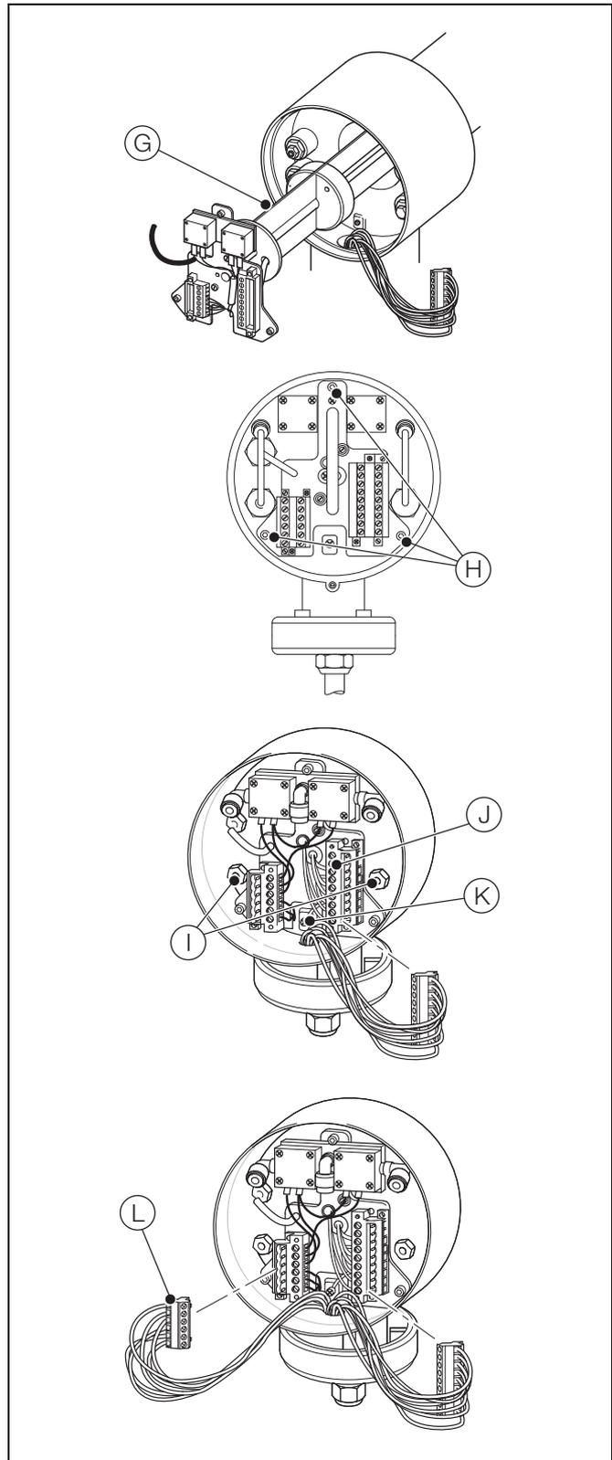
Fig. 5.17 Re-positioning the Inner Assembly and Making Terminal Plug Connections
