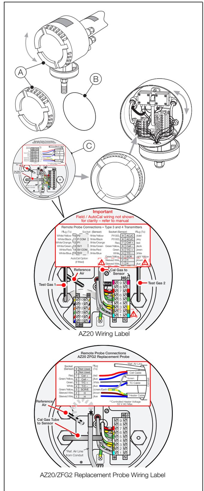
Fig. 5.3 Replacing the End Cap and Seal
