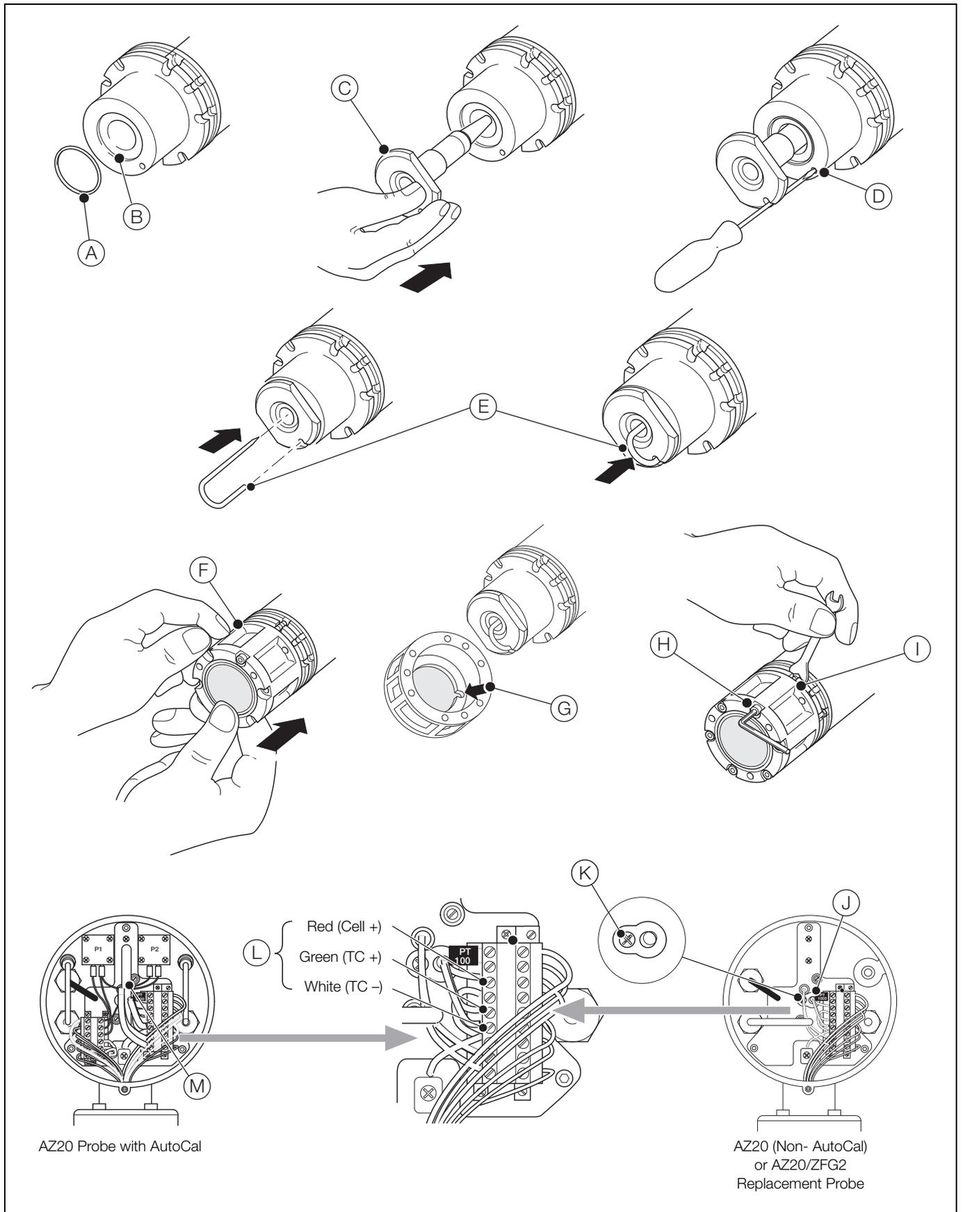
Fig. 5.6 Fitting a New C-ring and Cell
