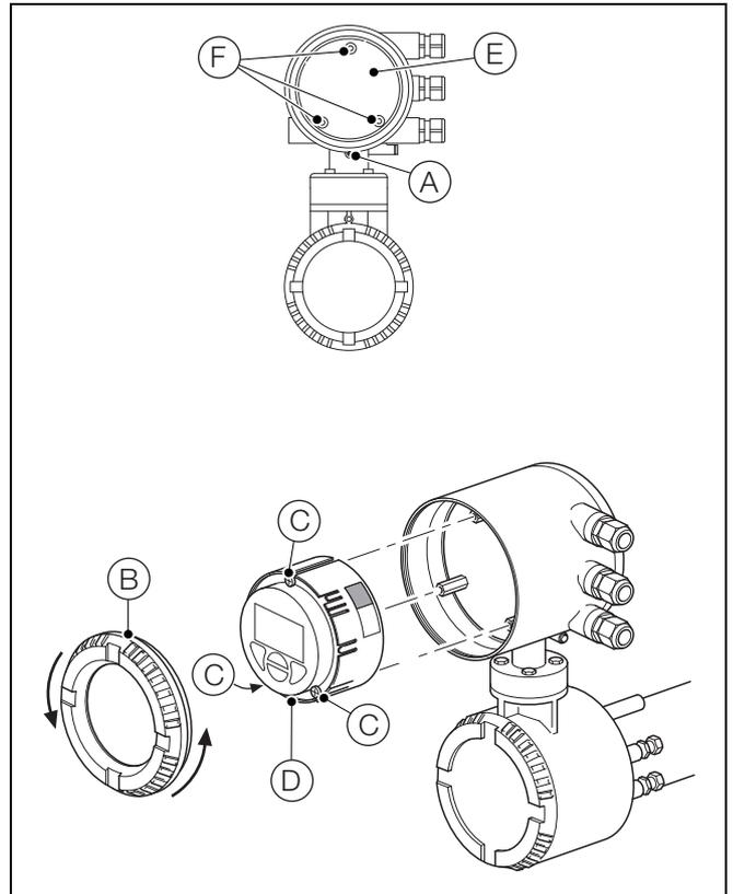
Fig. 6.2 Replacing the Cartridge on an Integral Transmitter
