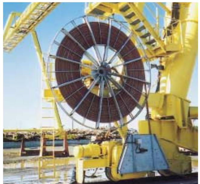
A Cavotec Specimas cable reel working at  $\pm 200$  m/min on a P&H log-handling crane for Federal Paper Board, in Augusta USA.
