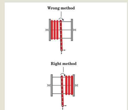
Figure 4. Winding of cable onto multi-spiral reel.
